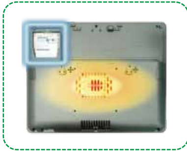
HDD isolated from main heat source on mother board
